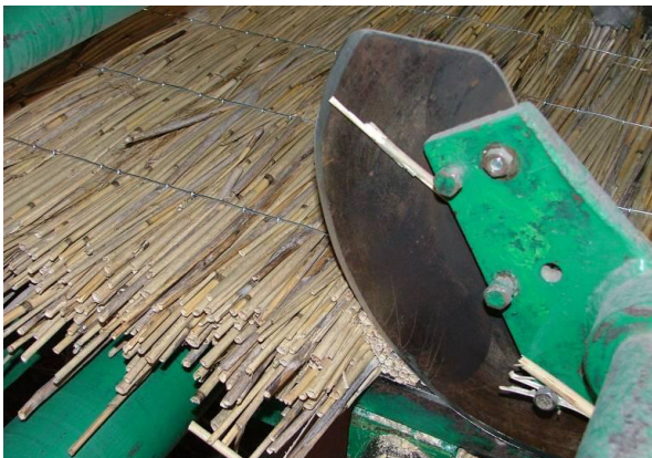
Fig. 2. Cutting of the ends of the reed board [2] Fig. 3. Cutting of the ends of the reed bundles [2]
